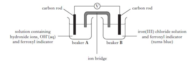
a) In beaker A hydroxide ions are converted into water molecules:
