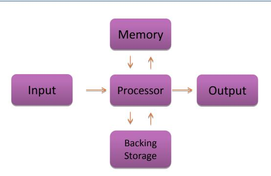
This is simple representation of how a computer works.
