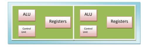
Now it is common for a CPU chip to have two, four, eight cores or more. A CPU with two cores is called 'dual' core and one with four cores is called 'quad core'. Each core can have its own internal cache to improve performance as well as shared cache within the CPU. Increasing the number of cores improves performance in two ways.
