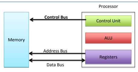
The Processor (CPU) has buses. These are multiple lines that connect the processor and main memory and used to transfer data and send signals between them.
